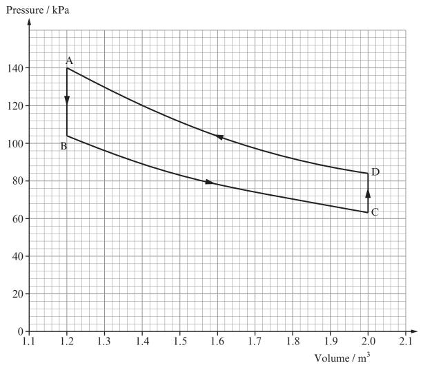
**BC** and **DA** are isotherms (the temperature along each of BC and DA is constant) and there are **49.3 mol** of ideal gas.
